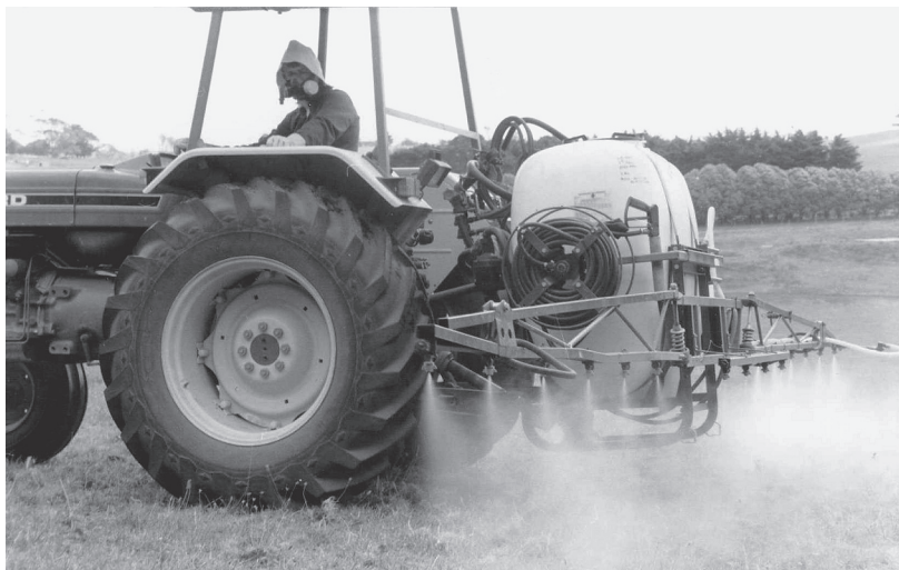
Figure 1. Incorrect sprayer settings that produce excessive fine droplets are one cause of drift.
